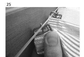
Hook all other screen hooks onto the ready tightened poly cord. Picture without 8 mm aluminium tubes
