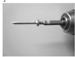
For installations in wooden structures, use wood screws
