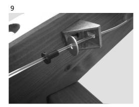
Pull the poly cord through the oval hole, then through the washer and finally through the plastic grommet. Pay attention to the direction on the plastic grommet
