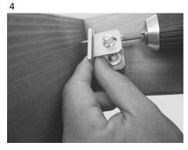
Install the wire-tightener and spacer plate. After the tip of the screw has pierced the aluminium, the thread will grab. **!ATTENTION!** Especially when using thin aluminium do not tighten too heavily
