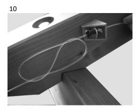
Tie the poly cord to a Flemish eight knot. Please do not knot in any other way because a secure hold can no longer be guaranteed then.
