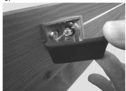
Push the covering cap heavily onto the support wire bracket
