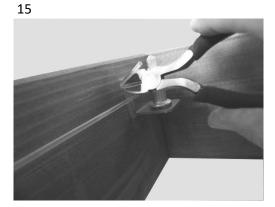
Remove the extra poly cord by the wire-tightener
