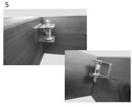
Picture on the left: the square bar to tighten points to the top. Picture on the right: the square bar to tighten points to the bottom
