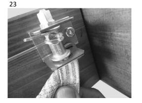
Screen hooks hooked into wiretightener
