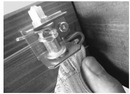
Pull the screen hooks on at the end of the sun screen, by the small pocket, toward the wire-tightener and hook it into the wire-tightener
