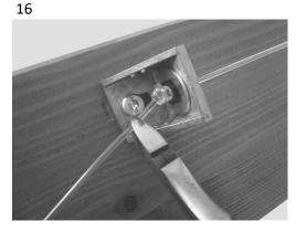
By the support wire bracket cut the extra poly cord with a approx. distance of 1,5 cm from the knot. If the end of the cord should stick up to the top, just twist it into the wiretightener
