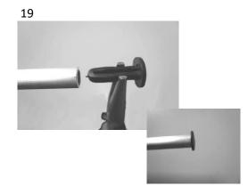
Put a plastic end-cap on one side of all 8 mm aluminium tubes. Use needlenose pliers for that. Alternatively you can insert those endcaps using a small hammer
