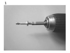
For installations in metal structures, use self-tapping drilling screw.
